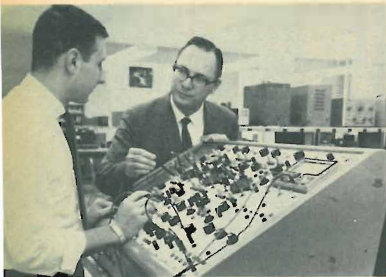
Design techniques are an important part of the technical institute student's training. In this photo an instructor checks out a student-designed circuit with transistor circuit synthesizer.
