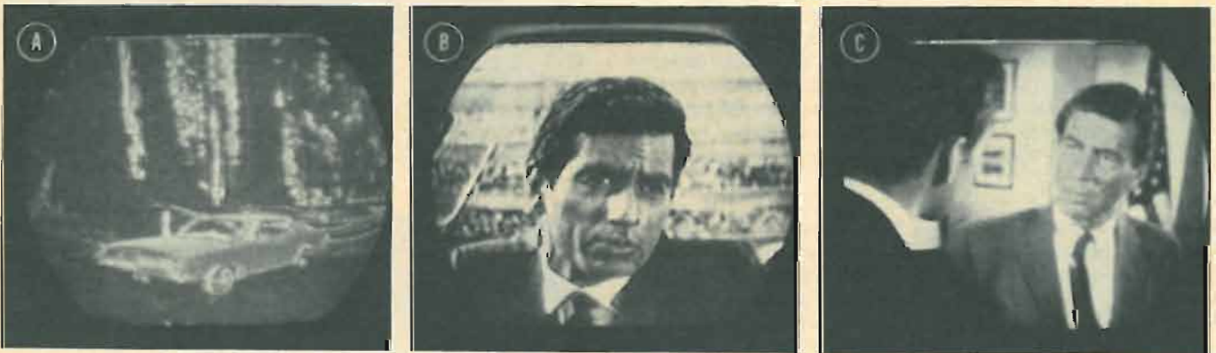
Fig. 1. (A) Severe beat interference. (B) Slight beat interference, (C) Properly tuned-in black-and-white picture.
