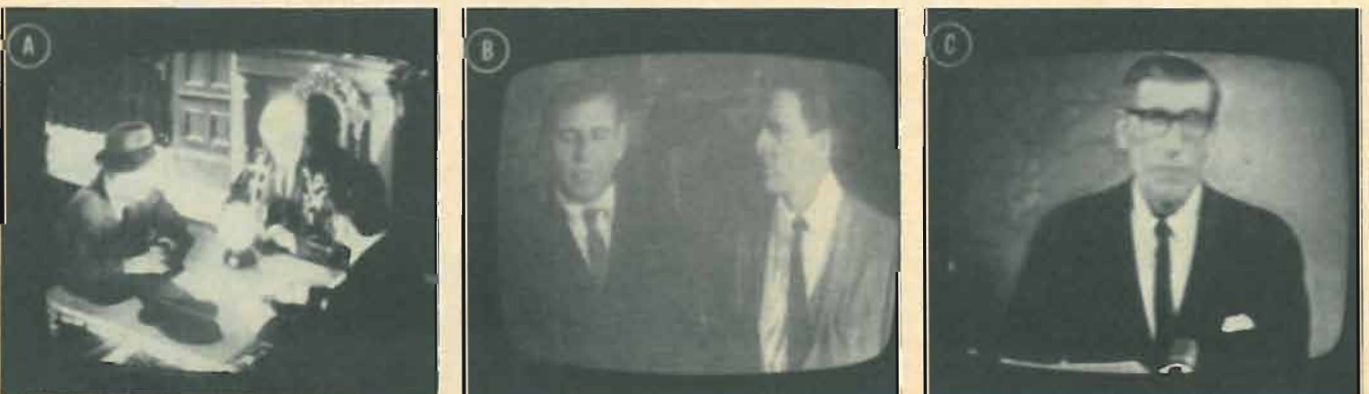
Fig. 2. (A) Excessive brightness and contrast. (B) Insufficient brightness and contrast. (C) The proper settings.
